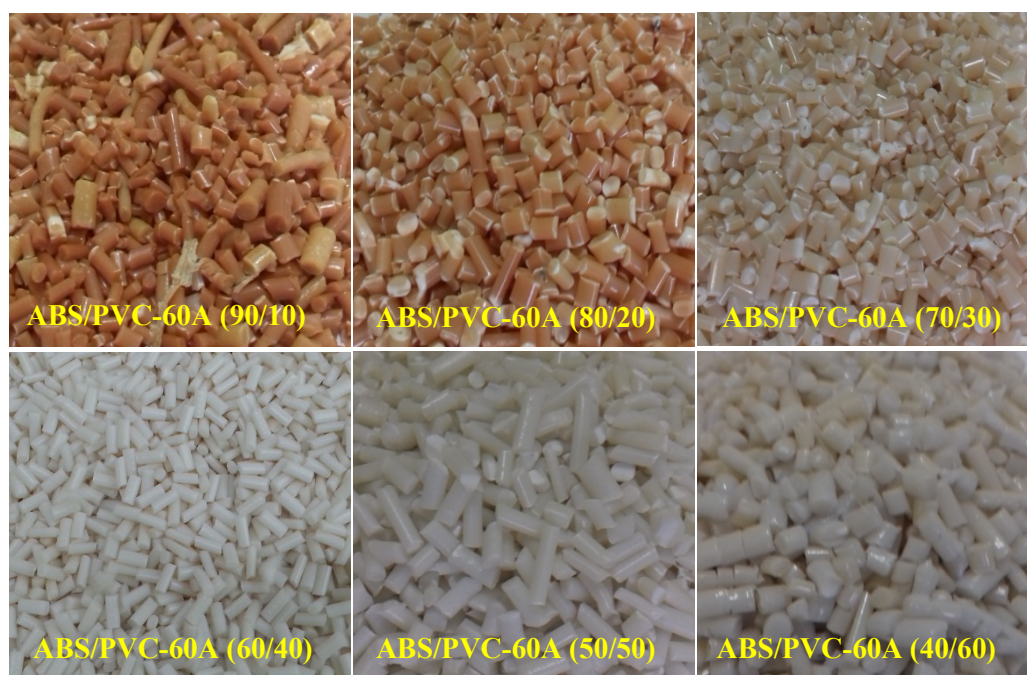
Figura 19: Misturas ABS/PVC-60A (90/10), ABS/PVC-60A (80/20), ABS/PVC-60A (70/30), ABS/PVC-60A (60/40), ABS/PVC-60A (50/50), ABS/PVC-60A (40/60), respectivamente.
